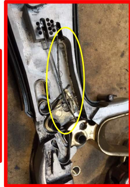
BREAKING/PINCHING OF CABLE SHEATHS
