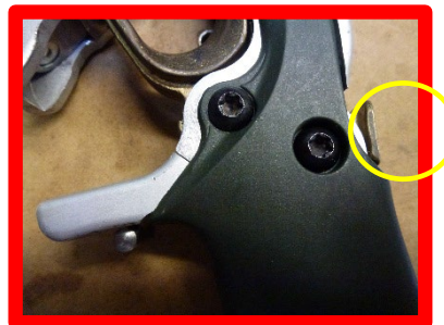
SCREW TOO TIGHT
