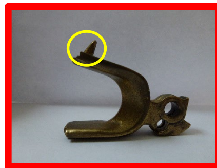
GUT OF U-HOOK BROKEN
