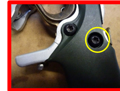
SCREW TOO TIGHT
